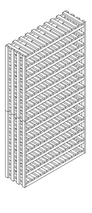
6. Anchor the racks to the wall using the recommended hardwares (not provided)
